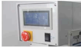
PLC Control Touch Screen Panel
