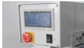
PLC Control Touch Screen Panel
